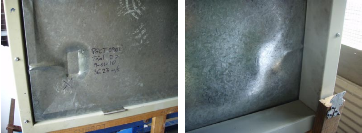
Figure 4: Door damage after Trial SU1
