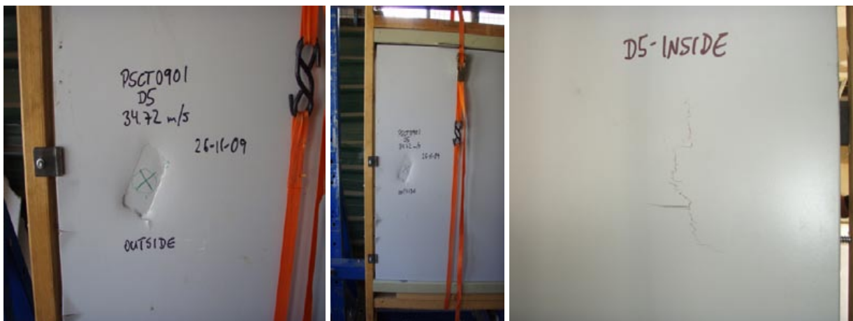
Figure 2: Door damage after Trial SS2
