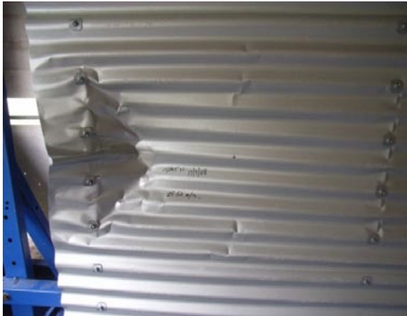
Figure 5: Cladding damage after Trials C7 (left) and C8 (right)
