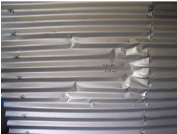
Figure 6: Cladding damage after Trial C9
