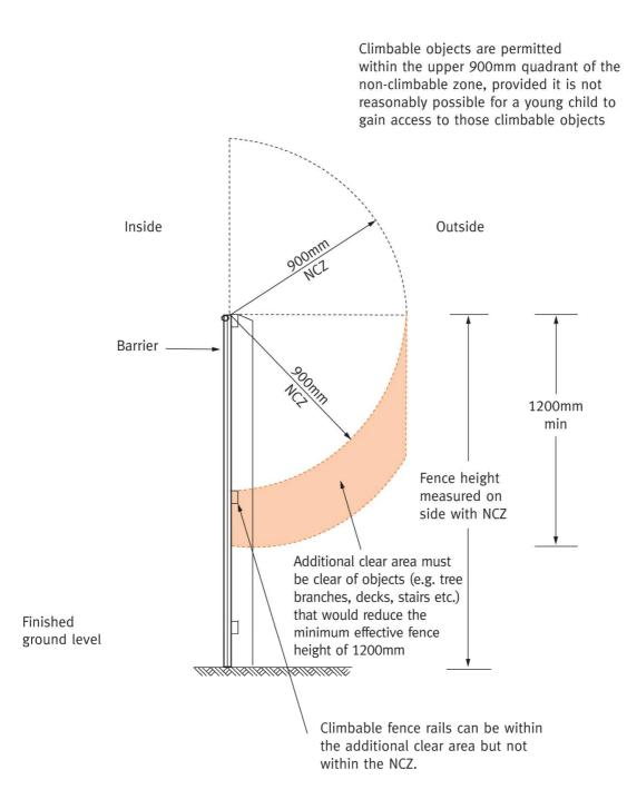
*Figure 12* Fence greater than 1200mm min high NCZ on outside *Acceptable*
