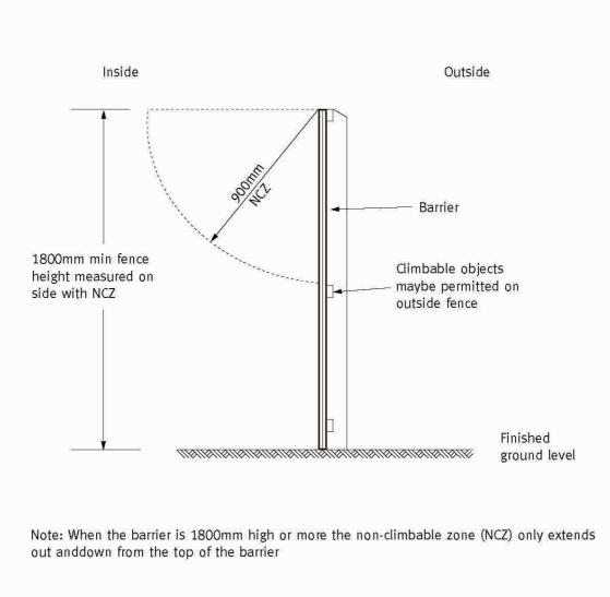
*Figure 10* 1800mm min high fence NCZ on inside *Acceptable*
