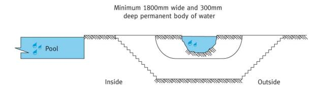
Figure 21 (b) Access provided under the permanent body of water (tunnel, pipe or service duct or the like)
