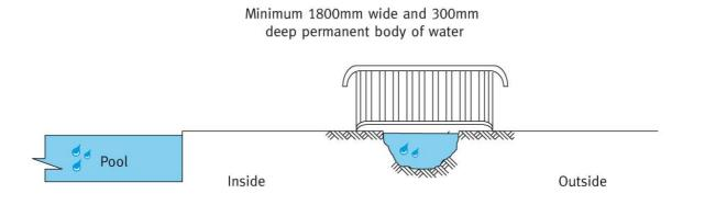
Figure 21 (a) Access provided over the permanent body of water (bridge, walkway or Pontoon or the like)
