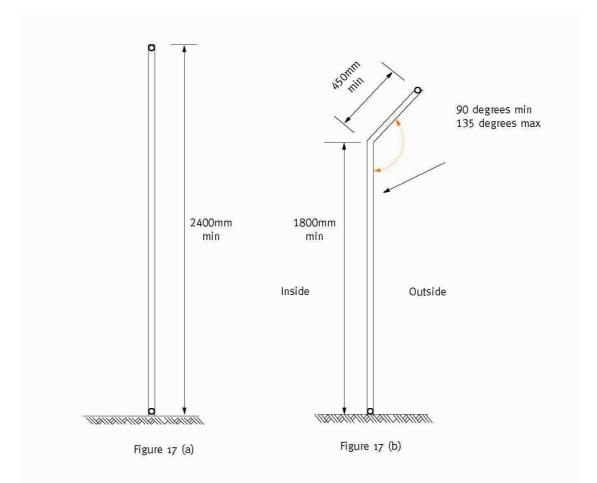
Note: Barriers using perforated material or mesh with apertures greater than 13mm but less than 100mm shall comply Figure 17(a) or (b) Barriers using mesh must include a strainer wire or rail at the top and bottom of the fencing In Figure 17(b) the cranked top shall have apertures less than 100mm
