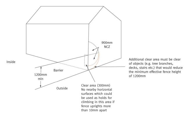
Note: The non-climbable zone (NCZ) continues in spherical form at the intersection of the pool barrier with the structure to the wall of the structure. The additional clear area continues in an arc past the intersection to the wall of the structure.
