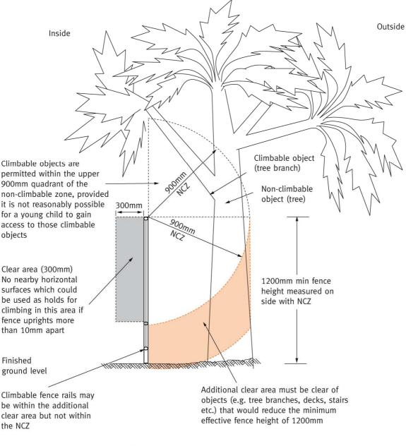
*Figure 9* 1200mm min high fence NCZ on outside *Acceptable*
