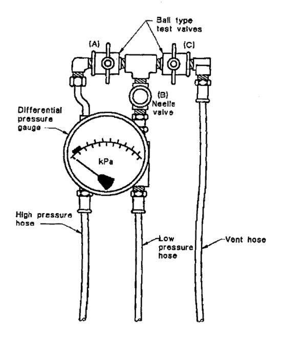
Figure 1 – Typical test kit apparatus
