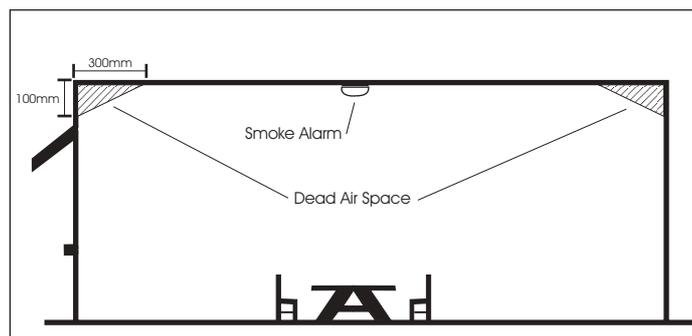
Figure 2: Illustration of the dead air space in the corner of rooms
