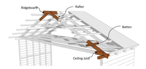
Picture: Minimal upgrade requirements to a pre-1980s roof structure.
