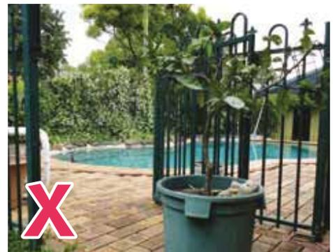
This gate is being held open by a pot plant, which could also be used to climb into the pool area and must be removed.
