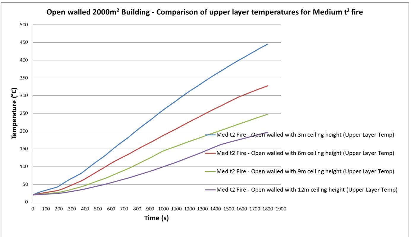
Figure 38: Smoke layer temperature for **Medium t<sup>2</sup> fire** within an open walled building with a floor area of 2000m<sup>2</sup>
