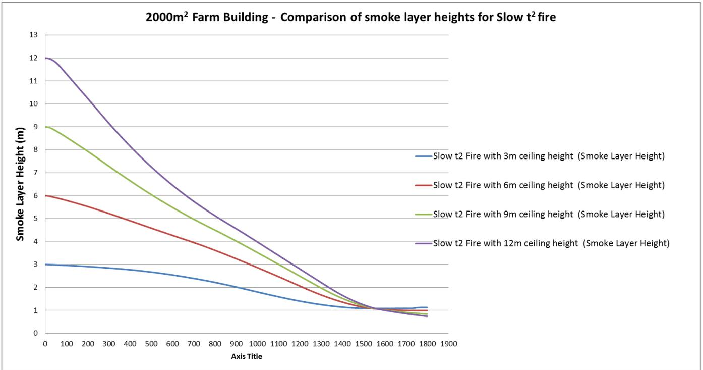
Figure 31: Smoke layer visibility for Slow t<sup>2</sup> fire within a floor area of 2000m<sup>2</sup>
