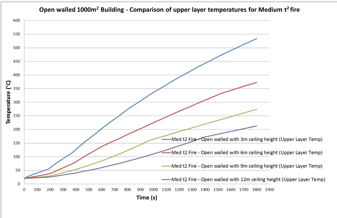
Figure 22: Smoke layer temperature for **Medium t<sup>2</sup> fire** within an open walled building with a floor area of 1000m<sup>2</sup>
