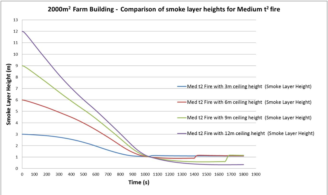
Figure 35: Smoke layer visibility for Medium t<sup>2</sup> fire within a floor area of 2000m<sup>2</sup>
