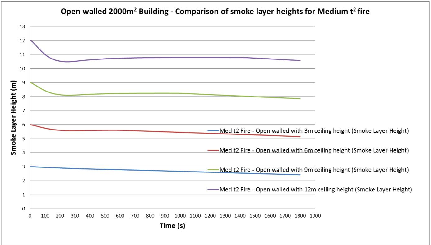
Figure 37: Smoke layer visibility for **Medium t<sup>2</sup> fire** within an open walled building with floor area of 2000m<sup>2</sup>
