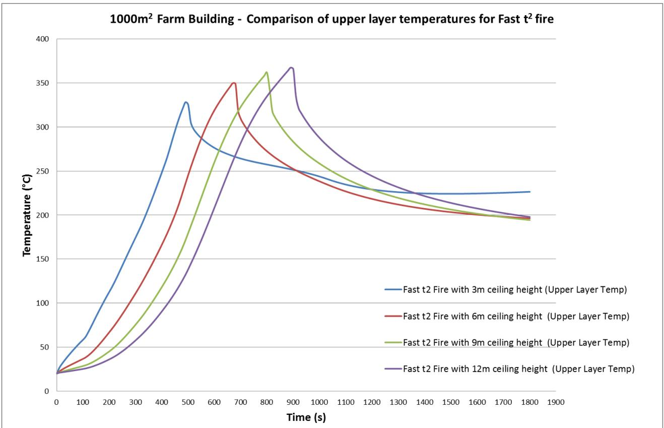
Figure 24: Smoke layer temperature for **Fast t<sup>2</sup> fire** within a floor area of 1000m<sup>2</sup>
