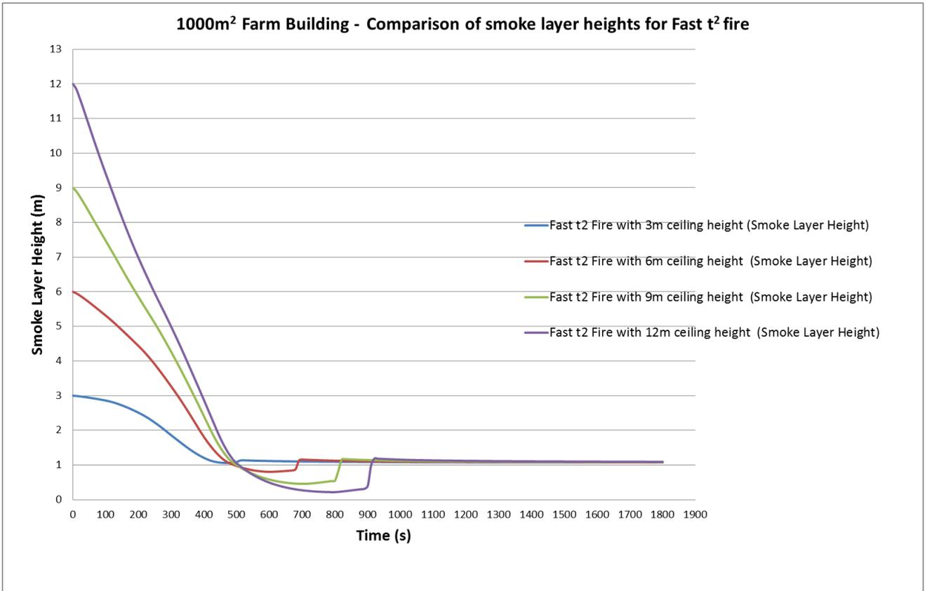
Figure 23: Smoke layer visibility for **Fast t<sup>2</sup> fire** within a floor area of 1000m<sup>2</sup>
