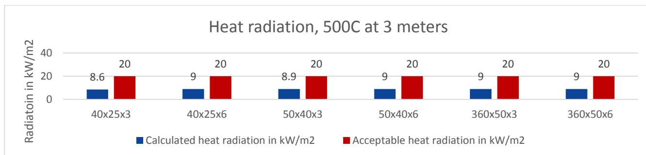
Figure 2: Heat radiation, 500 °C at 3 meters
