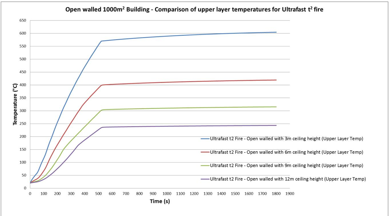
Figure 30: Smoke layer temperature for Ultrafast t<sup>2</sup> fire within an open walled building with floor area of 1000m<sup>2</sup>
