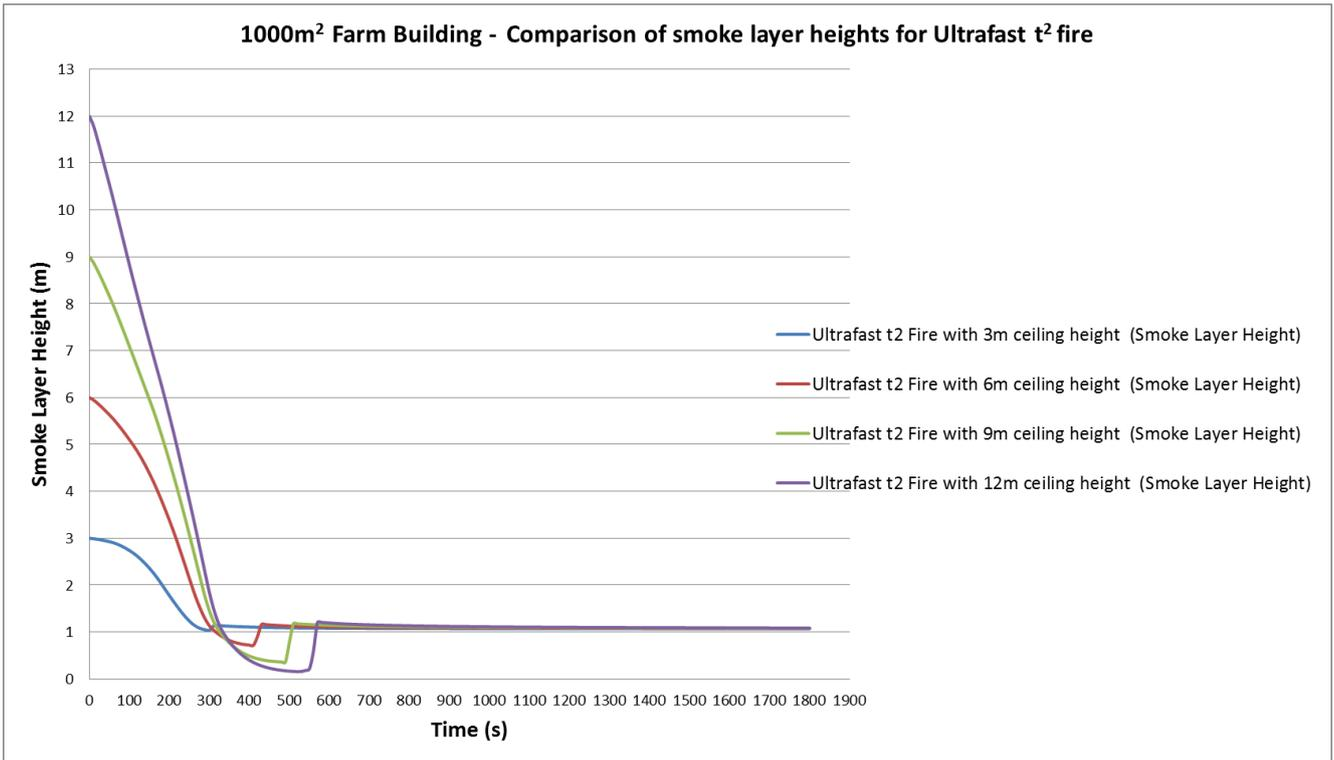
Figure 27: Smoke layer visibility for Ultrafast t<sup>2</sup> fire within a floor area of 1000m<sup>2</sup>
