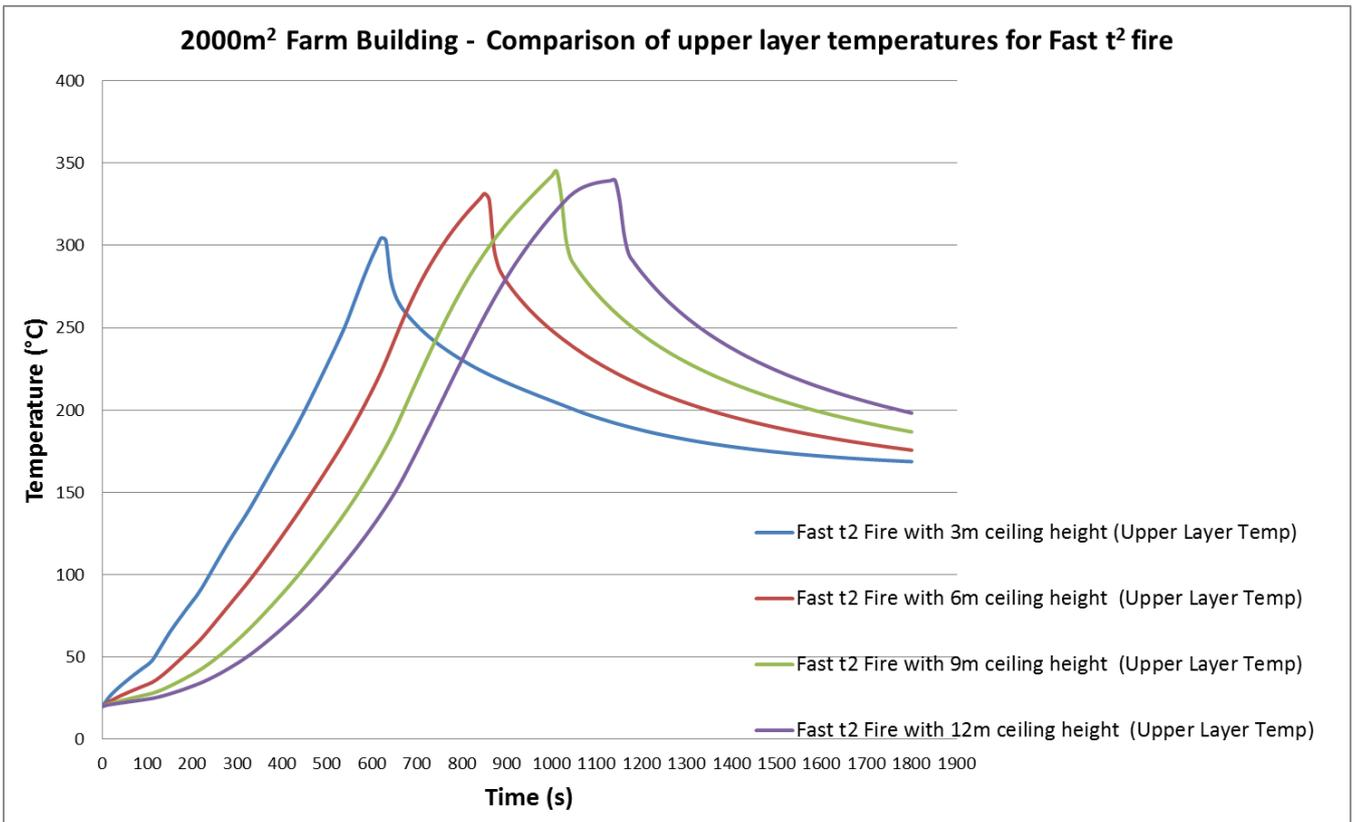
Figure 40: Smoke layer temperature for **Fast t<sup>2</sup> fire** within a floor area of 2000m<sup>2</sup>
