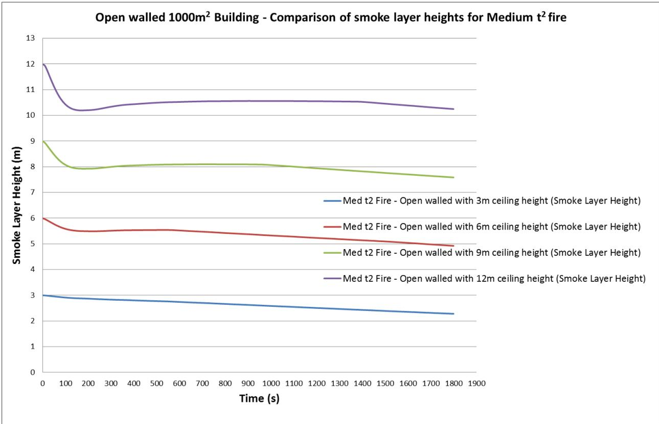
Figure 21: Smoke layer visibility for **Medium t<sup>2</sup> fire** within an open walled building with floor area of 1000m<sup>2</sup>
