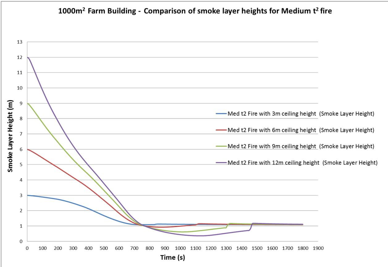
Figure 19: Smoke layer visibility for Medium t<sup>2</sup> fire within a floor area of 1000m<sup>2</sup>
