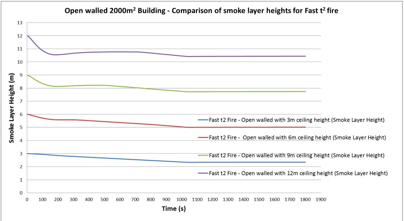
Figure 41: Smoke layer visibility for **Fast t<sup>2</sup> fire** within an open walled building with floor area of 2000m<sup>2</sup>
