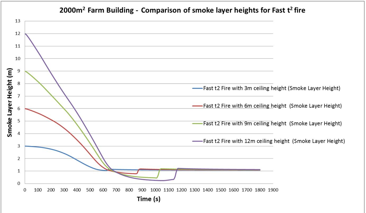
Figure 39: Smoke layer visibility for **Fast t<sup>2</sup> fire** within a floor area of 2000m<sup>2</sup>
