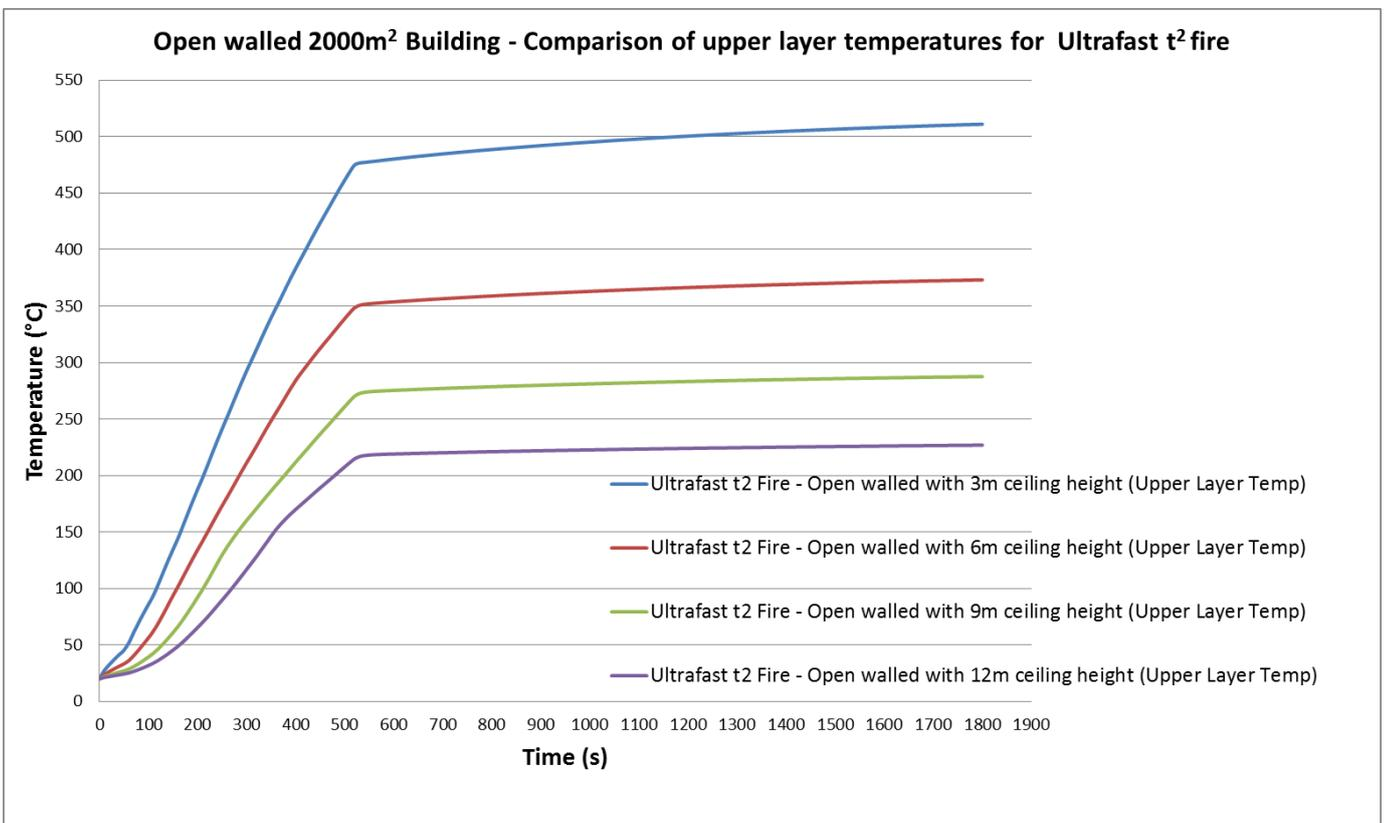
Figure 46: Smoke layer temperature for Ultrafast t<sup>2</sup> fire within an open walled building with floor area of 2000m<sup>2</sup>
