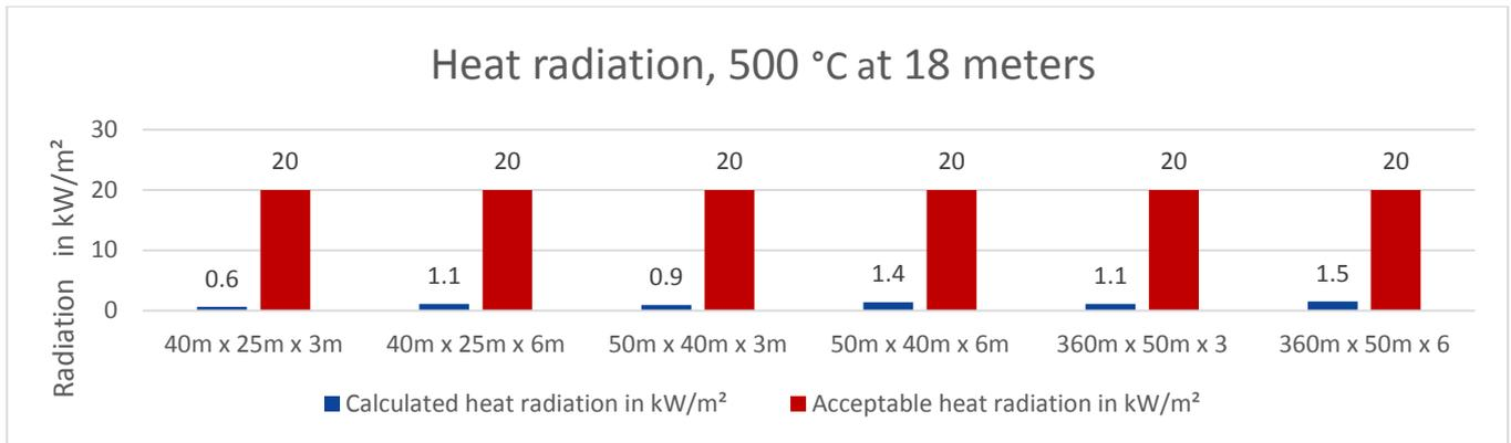
Figure 6: Heat radiation, 500°C at 18 meters
