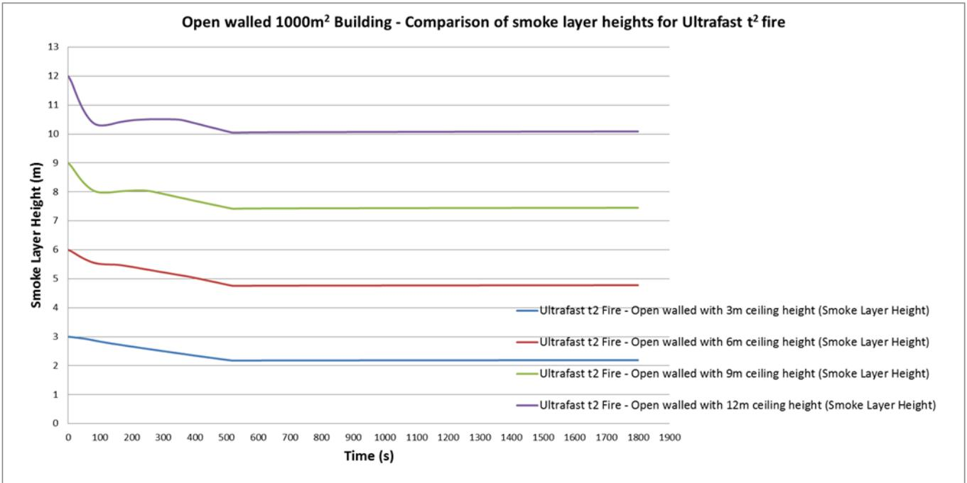
Figure 29: Smoke layer visibility for Ultrafast t<sup>2</sup> fire within an open walled building with floor area of 1000m<sup>2</sup>
