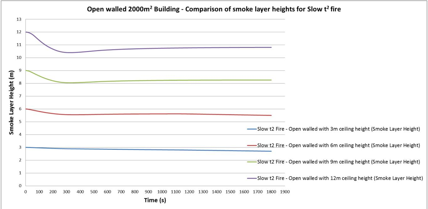
Figure 33: Smoke layer visibility for Slow t<sup>2</sup> fire within an open walled building with floor area of 2000m<sup>2</sup>
