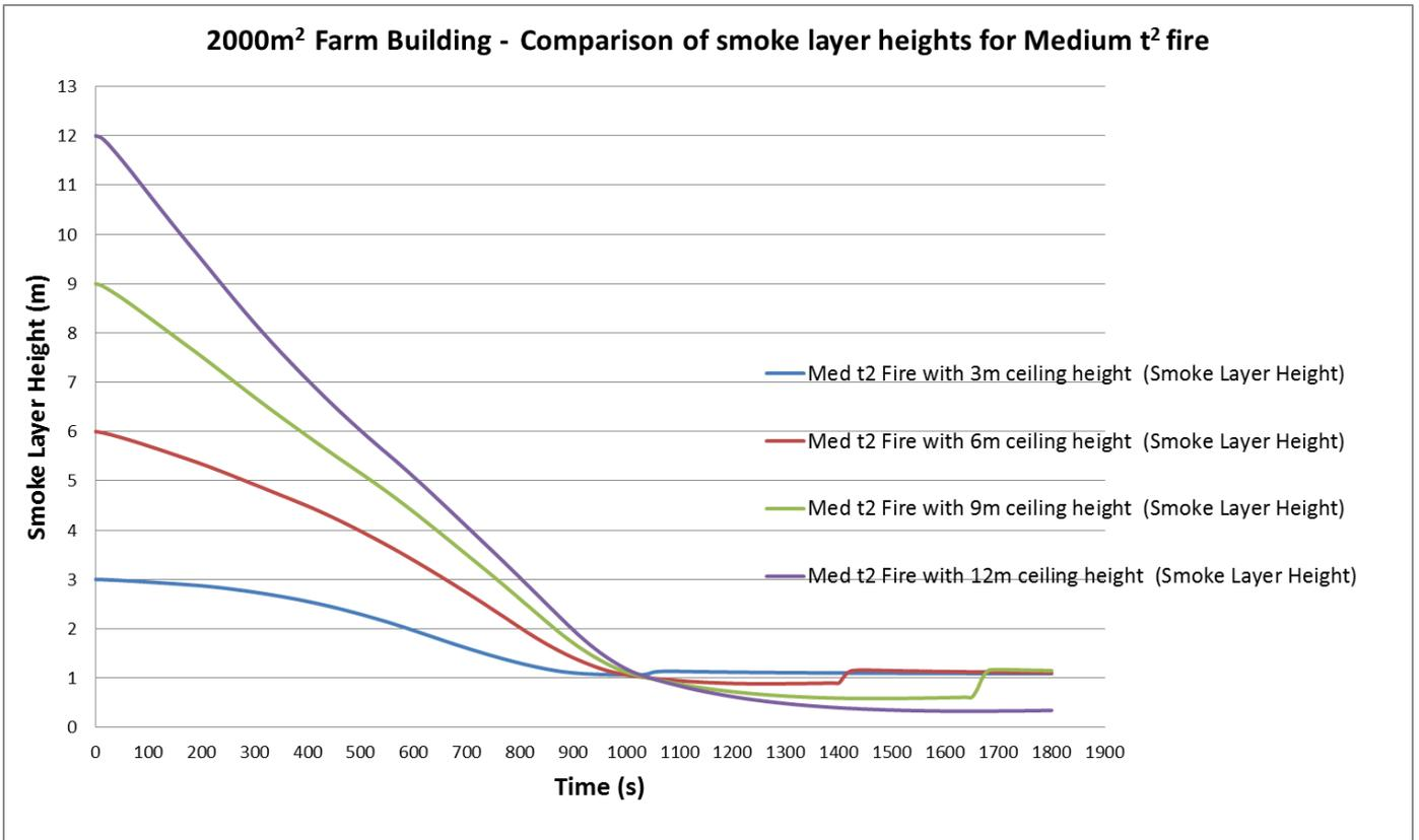
Figure 49: Smoke layer visibility for Medium t<sup>2</sup> fire within a floor area of 2000m<sup>2</sup>
