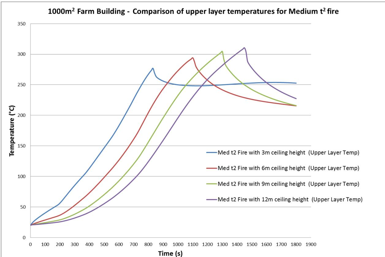
Figure 20: Smoke layer temperature for **Medium t<sup>2</sup> fire** within a floor area of 1000m<sup>2</sup>
