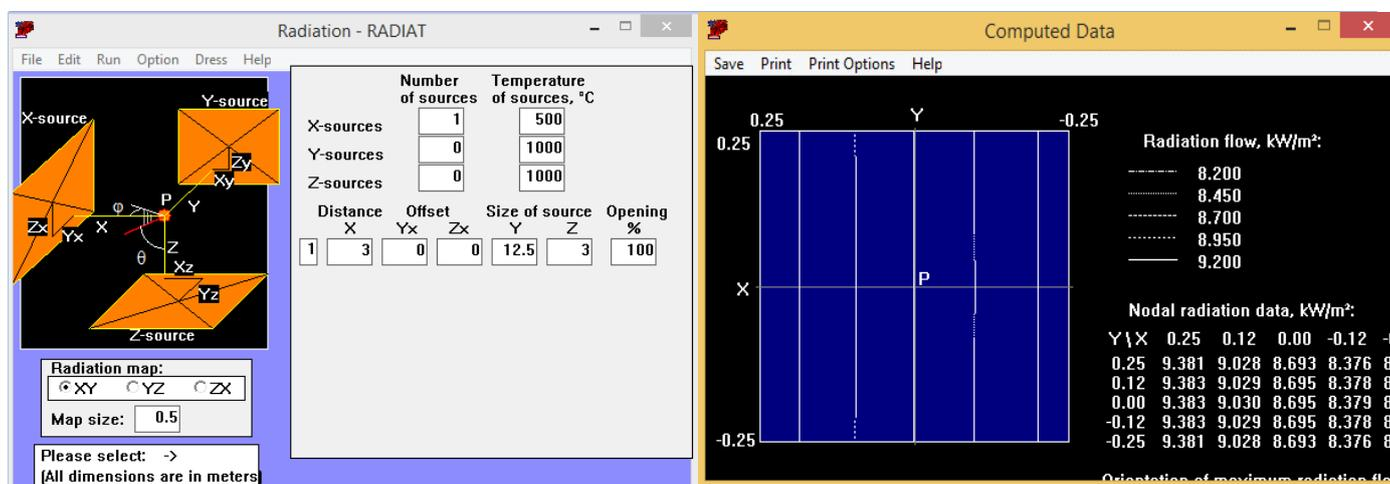
Figure 1: Sample radiation calculation using FIREWIND Program
