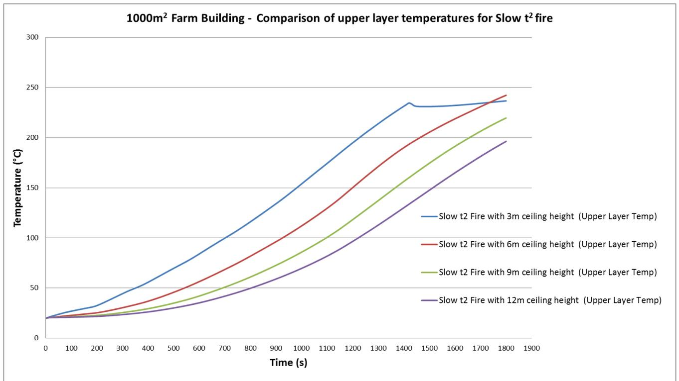
Figure 16: Smoke layer temperature for Slow t<sup>2</sup> fire within a floor area of 1000m<sup>2</sup>
