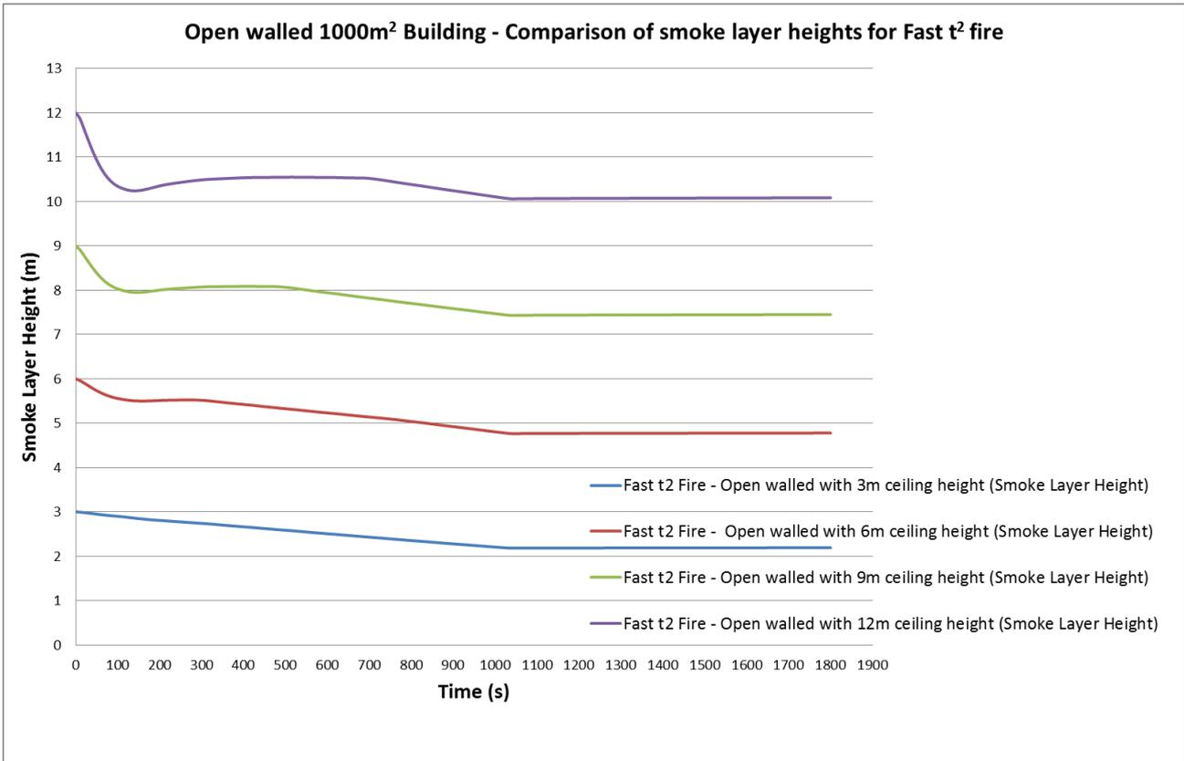
Figure 25: Smoke layer visibility for **Fast t<sup>2</sup> fire** within an open walled building with floor area of 1000m<sup>2</sup>
