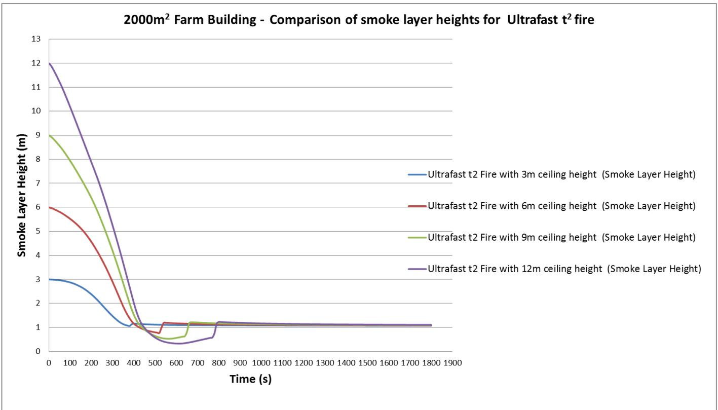
Figure 51: Smoke layer visibility for Ultrafast t<sup>2</sup> fire within a floor area of 2000m<sup>2</sup>
