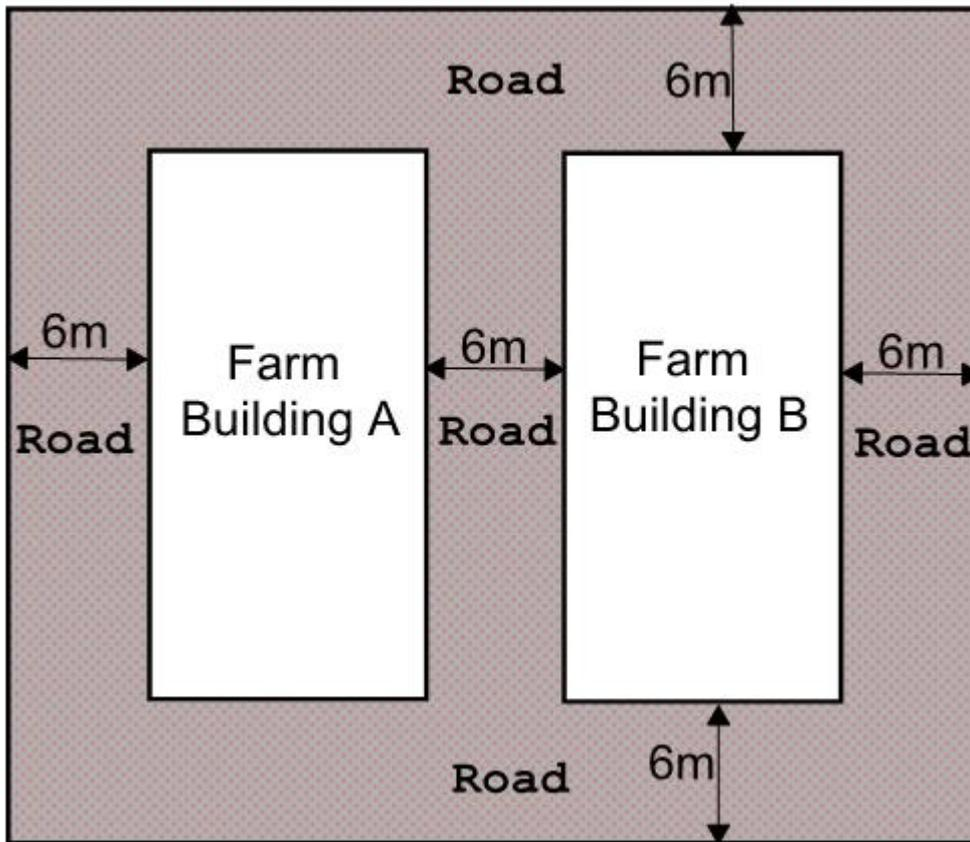
**Figure 12: Minimum separation distance of 6m would be necessary to minimise the risk of fire spread**
