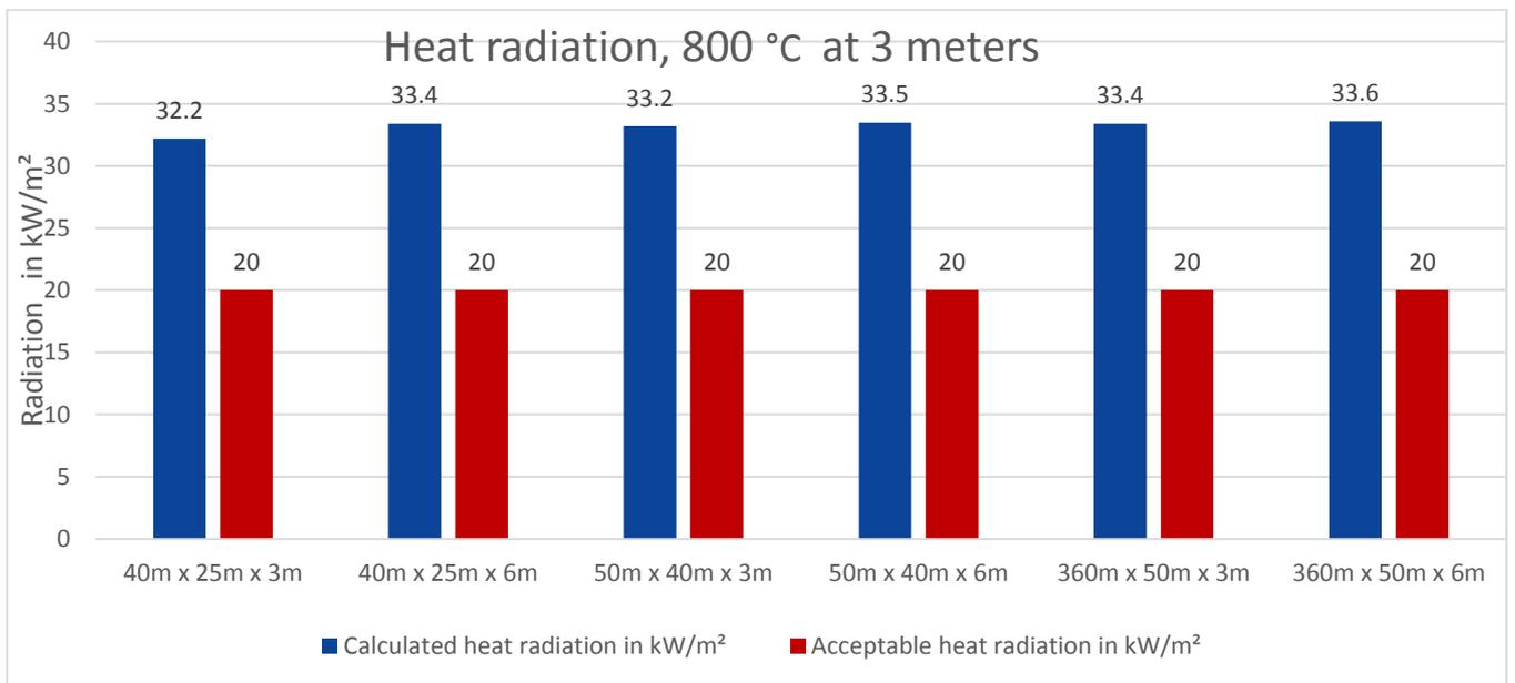
Figure 7: Heat radiation, 800°C at 3 meters
