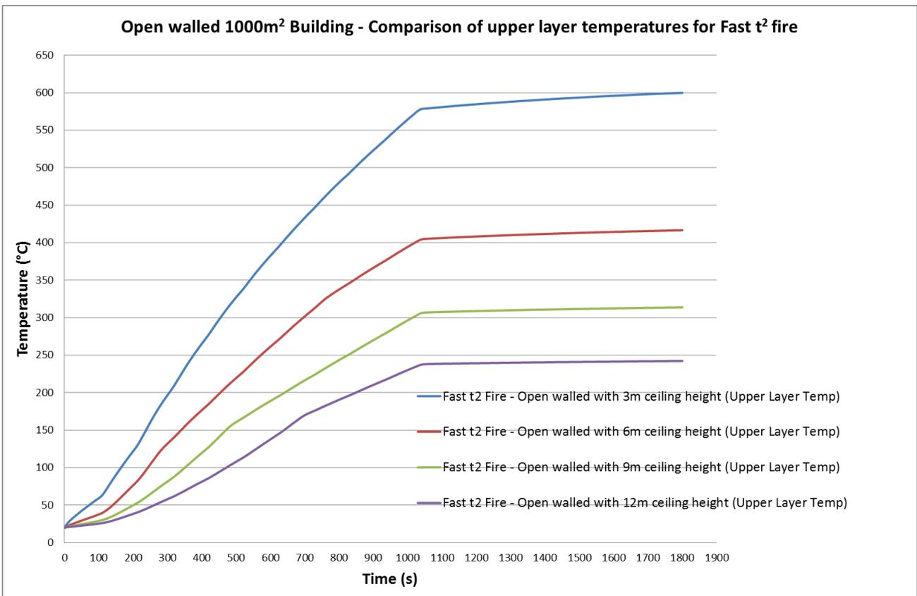
Figure 26: Smoke layer temperature for **Fast t² fire** within an open walled building with a floor area of 1000m²
