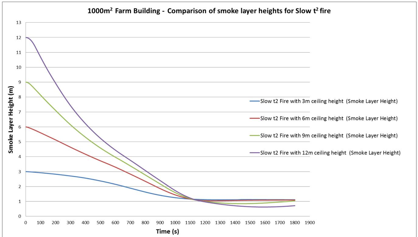
Figure 15: Smoke layer visibility for Slow t<sup>2</sup> fire within a floor area of 1000m<sup>2</sup>
