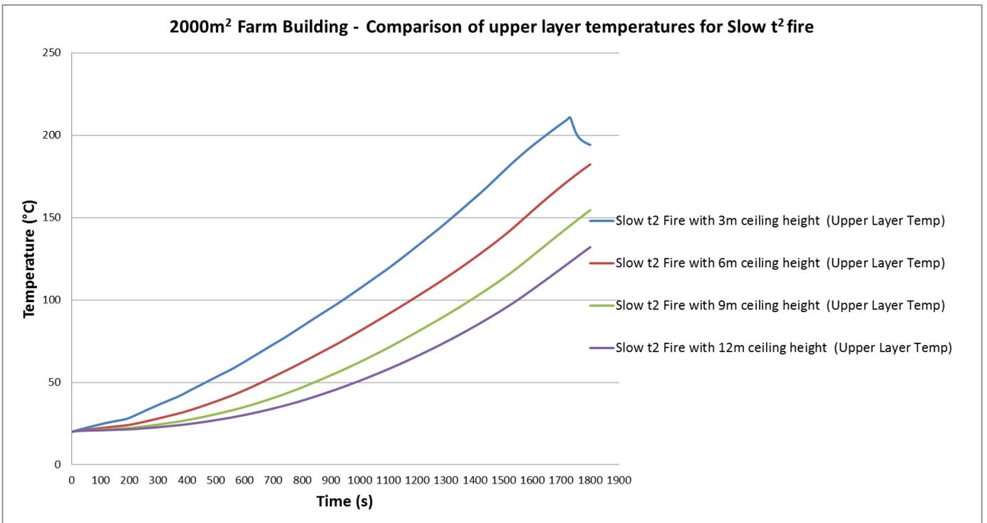
Figure 32: Smoke layer temperature for Slow t<sup>2</sup> fire within a floor area of 2000m<sup>2</sup>
