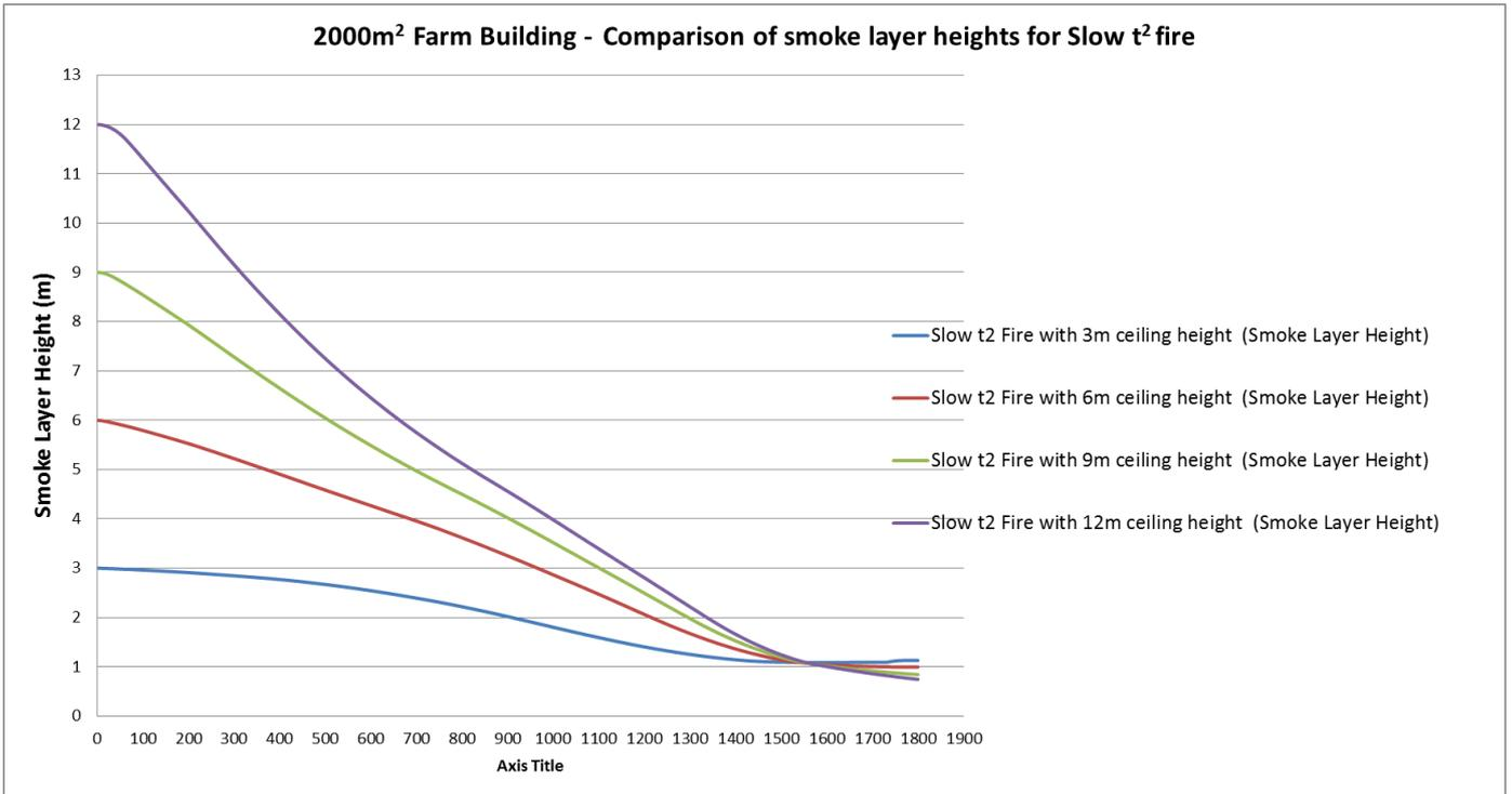
Figure 48: Smoke layer visibility for Slow t<sup>2</sup> fire within a floor area of 2000m<sup>2</sup>
