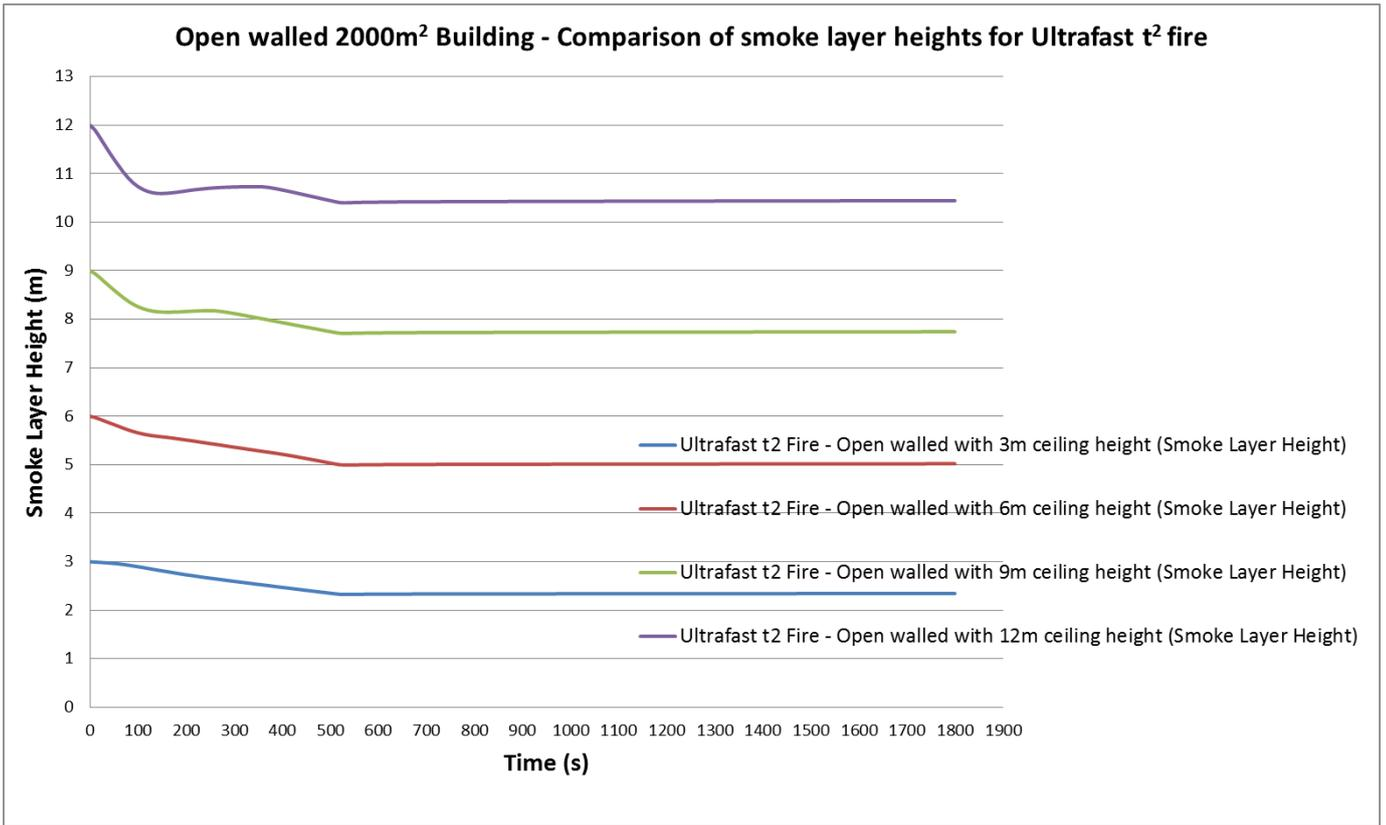
Figure 45: Smoke layer visibility for Ultrafast t<sup>2</sup> fire within an open walled building with floor area of 2000m<sup>2</sup>
