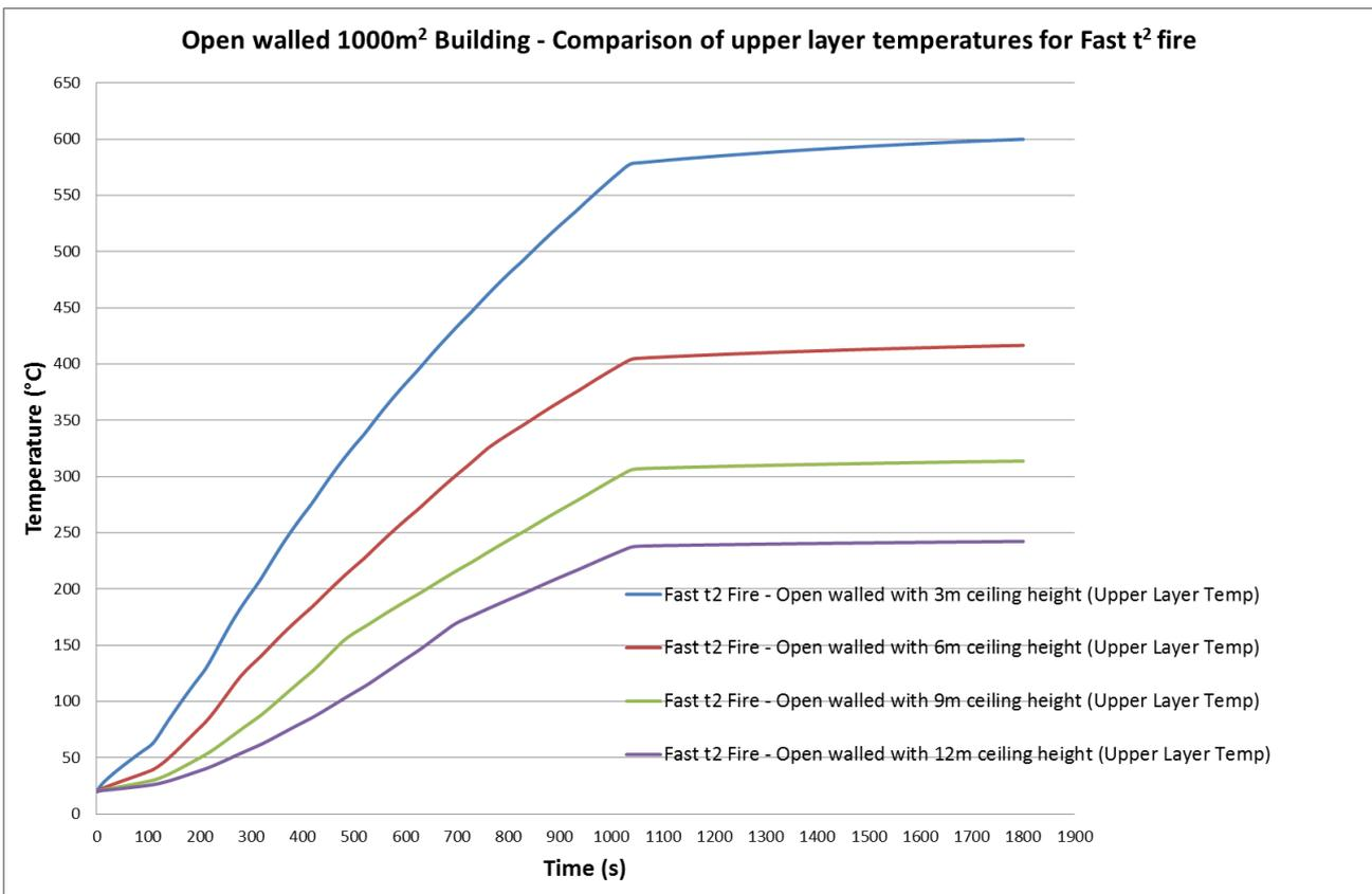
Figure 26: Smoke layer temperature for **Fast t<sup>2</sup> fire** within an open walled building with a floor area of 1000m<sup>2</sup>
