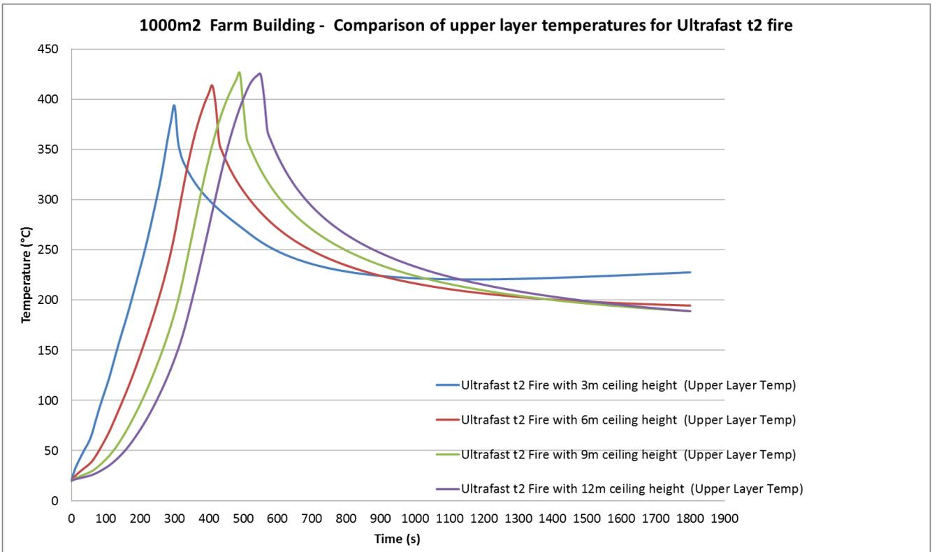
Figure 28: Smoke layer temperature for Ultrafast t<sup>2</sup> fire within a floor area of 1000m<sup>2</sup>
