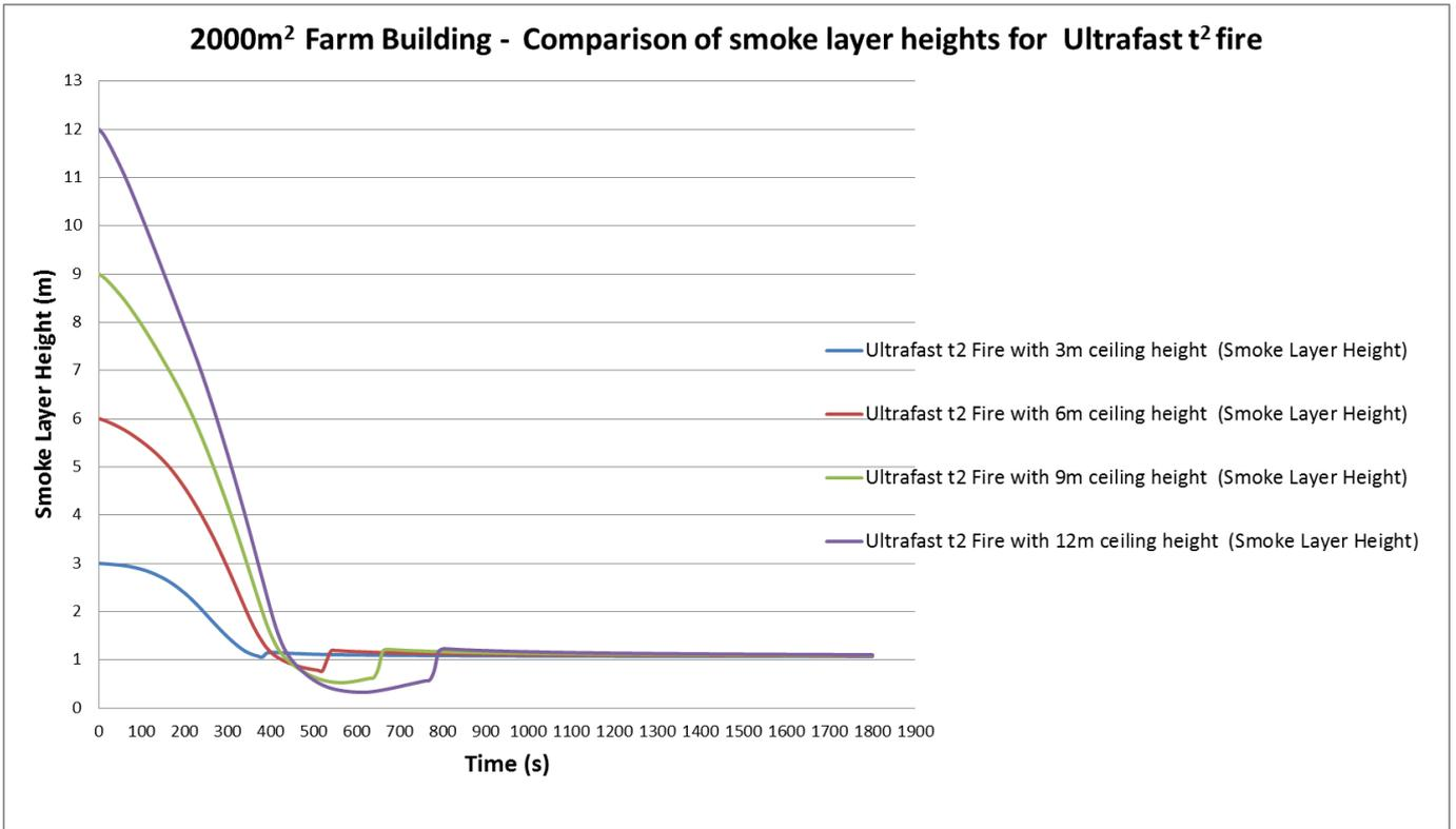
Figure 43: Smoke layer visibility for Ultrafast t<sup>2</sup> fire within a floor area of 2000m<sup>2</sup>
