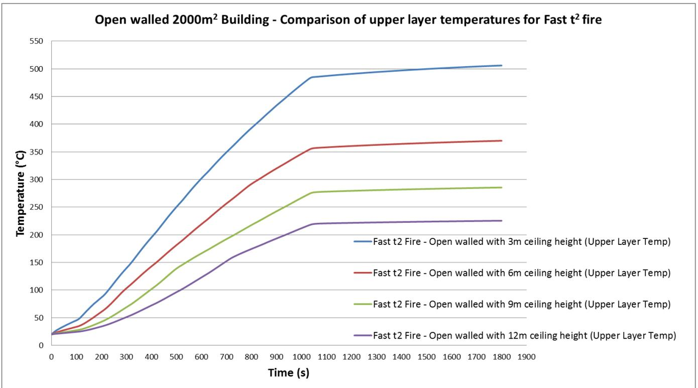
Figure 42: Smoke layer temperature for **Fast t<sup>2</sup> fire** within an open walled building with a floor area of 2000m<sup>2</sup>
