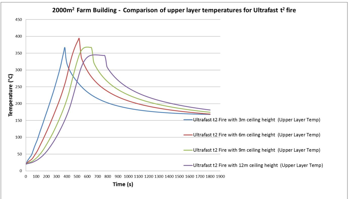
Figure 44: Smoke layer temperature for Ultrafast t<sup>2</sup> fire within a floor area of 2000m<sup>2</sup>
