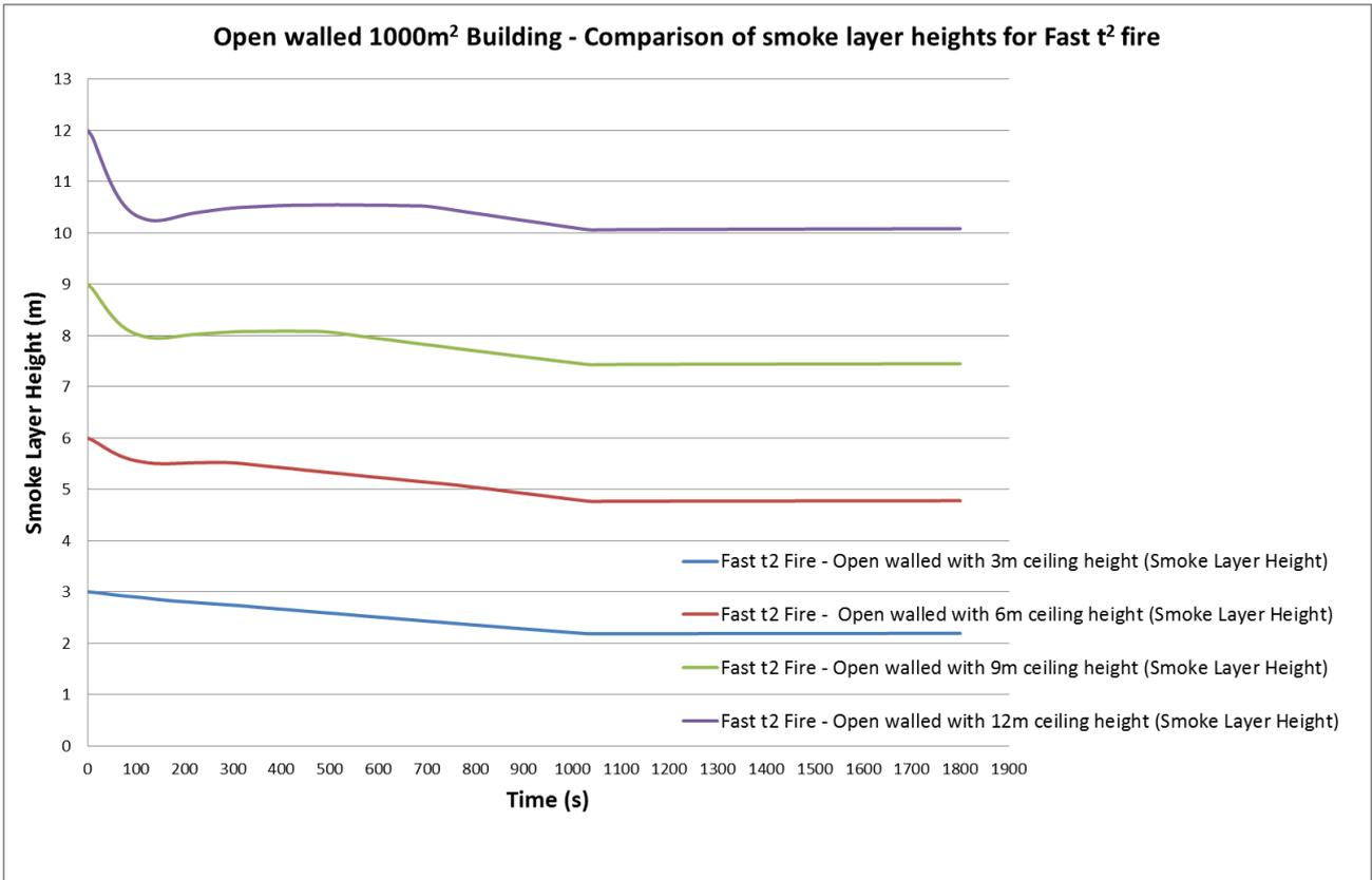
Figure 25: Smoke layer visibility for **Fast t² fire** within an open walled building with floor area of 1000m²
