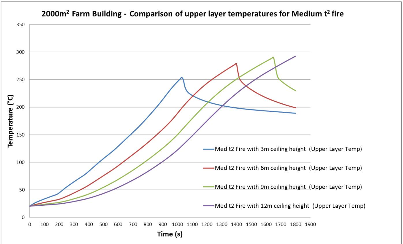
Figure 36: Smoke layer temperature for Medium t<sup>2</sup> fire within a floor area of 2000m<sup>2</sup>
