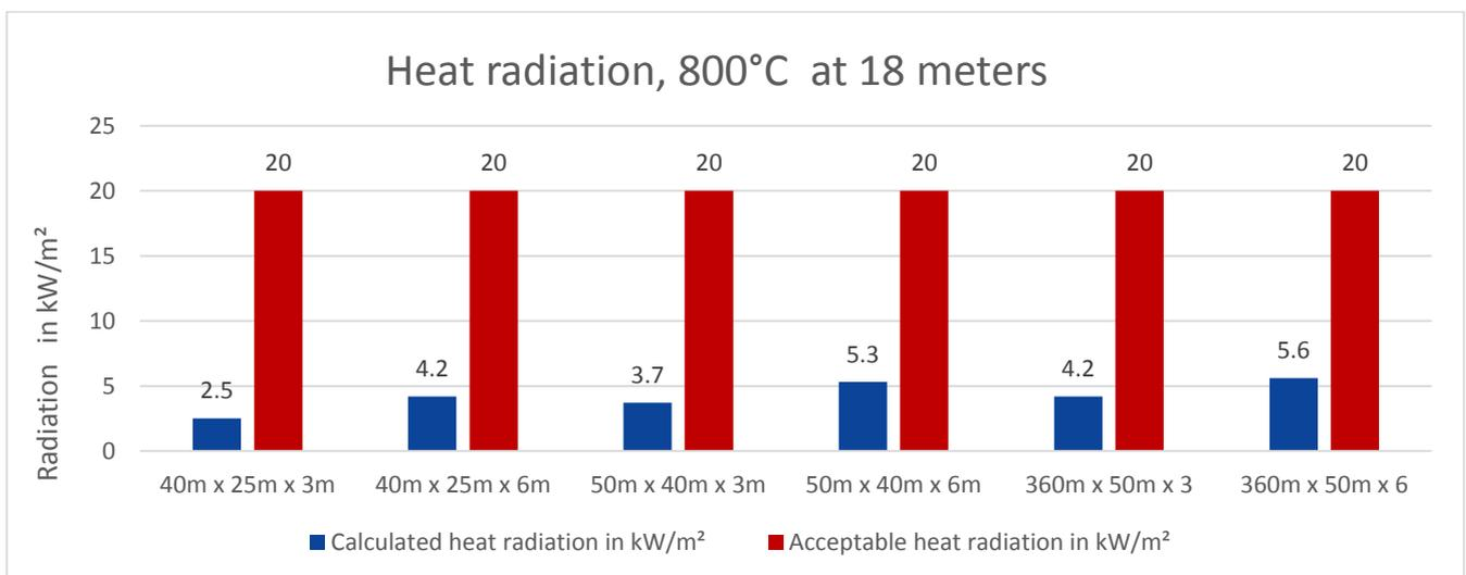
**Figure 11: Heat radiation, 800°C at 18 meters**
