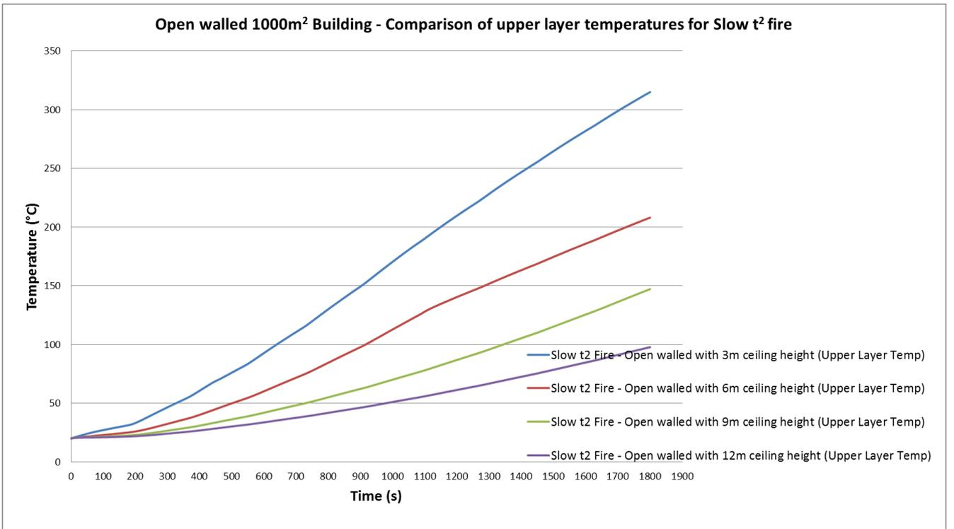
Figure 18: Smoke layer temperature for **Slow t<sup>2</sup> fire** within an open walled building with a floor area of 1000m<sup>2</sup>
