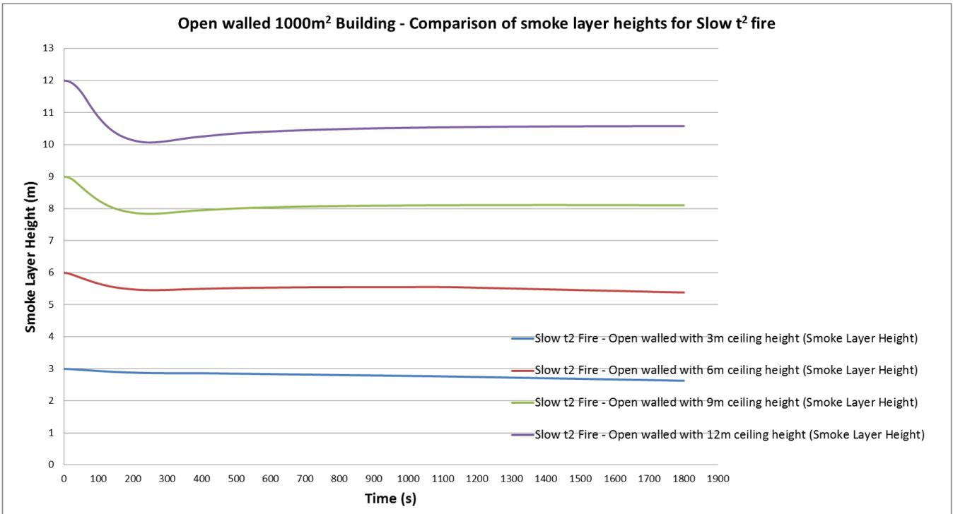
Figure 17: Smoke layer visibility for **Slow t<sup>2</sup> fire** within an open walled building with floor area of 1000m<sup>2</sup>
