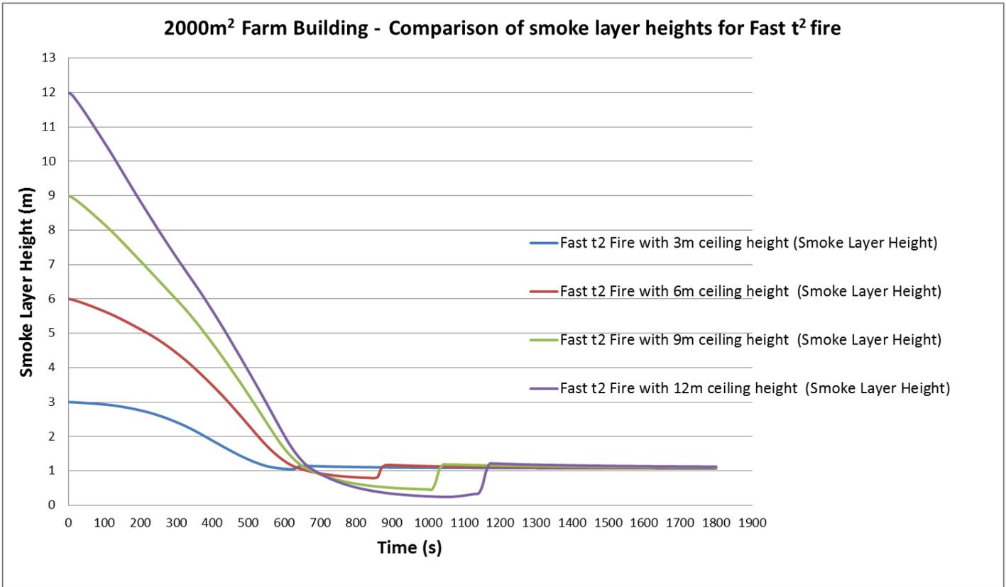
Figure 50: Smoke layer visibility for Fast t<sup>2</sup> fire within a floor area of 2000m<sup>2</sup>
