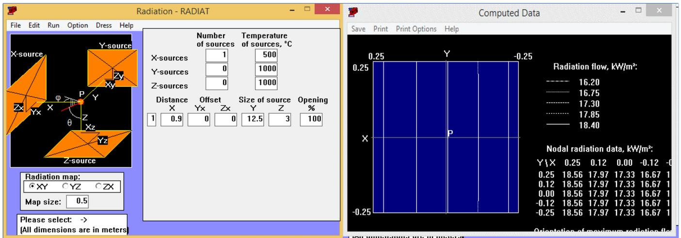
Figure 56: Radiation calculation using FIREWIND Program
