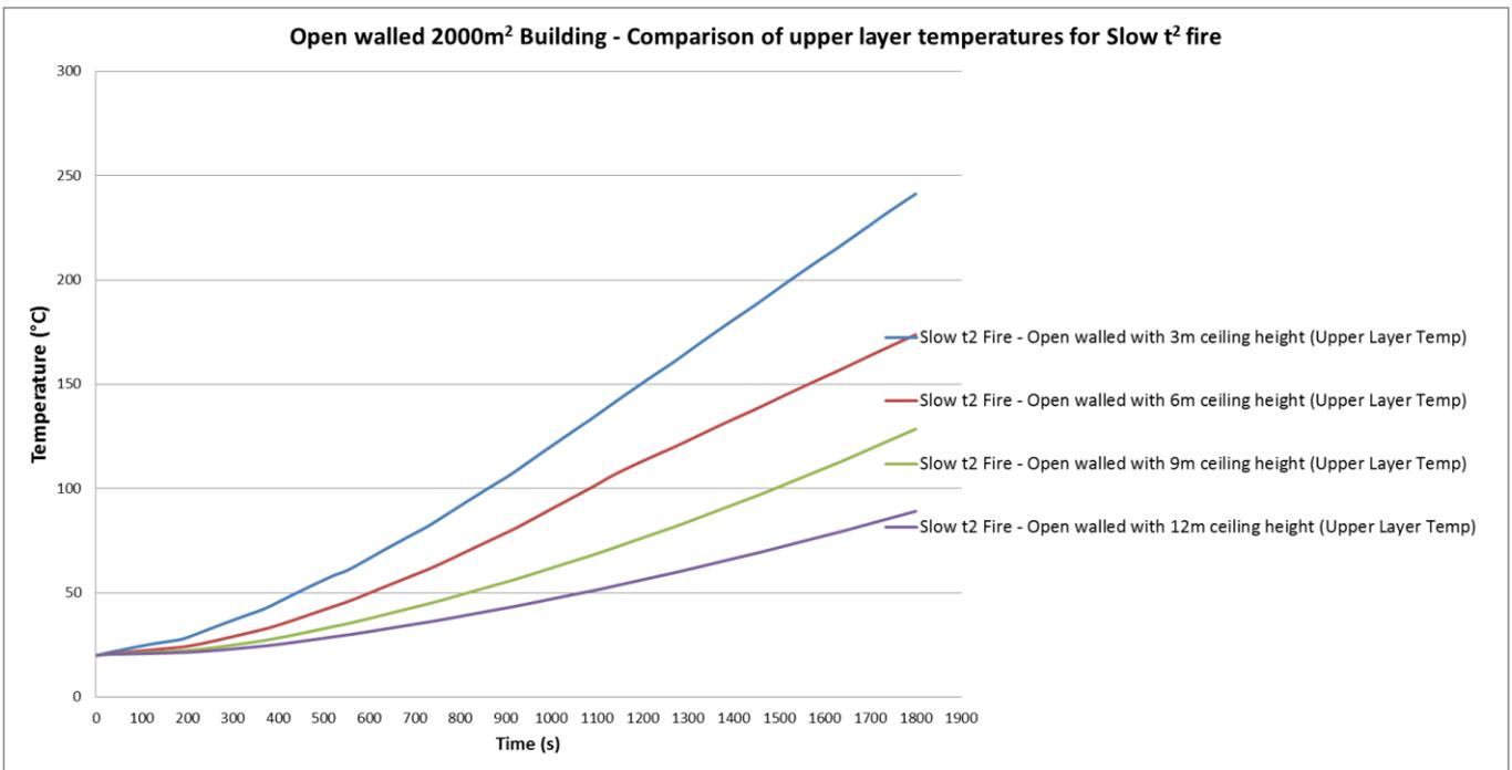
Figure 34: Smoke layer temperature for Slow t<sup>2</sup> fire within an open walled building with a floor area of 2000m<sup>2</sup>
