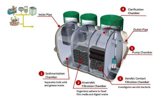
FujiClean ACE is designed to treat all household wastewater from the kitchen, bathroom, toilet and laundry area and is capable of producing Advanced Secondary Quality Effluent as specified below. The daily design flow rate of FujiClean ACE is 1,200 L/day.
