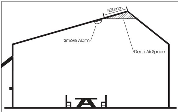
Figure 3: Illustration of the dead air space at the peak of sloped ceilings
